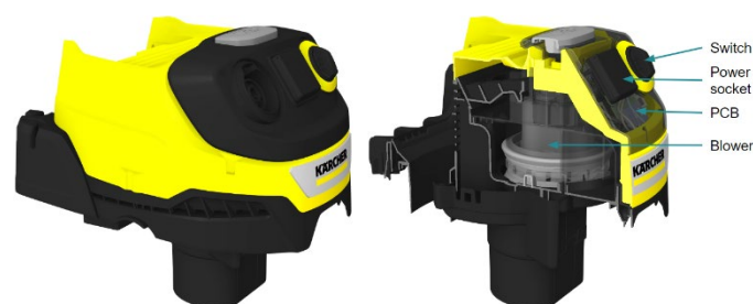
Figure 4 Illustration of a Kärcher WD6 wet and dry vacuum cleaner head, with a depiction of the main electrical parts.
