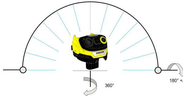
Figure 2 Illustrative depiction of the test rig for the IPX4 case.
