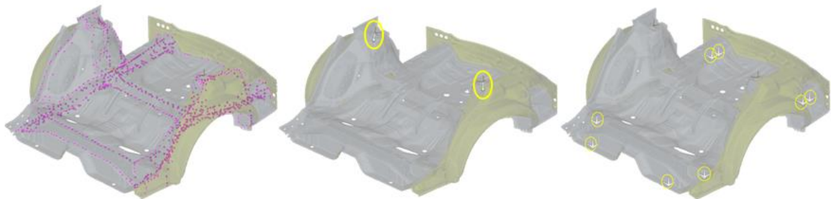
Fig. 1 a) Spot welds of the model, b) Applied forces, c) Boundary conditions
